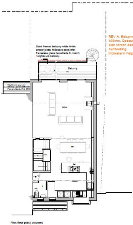
REV A: Balcony reduced in depth by 150mm. Opaque high level (1.8m from FF) side screen added to prevent sideways overlooking.
