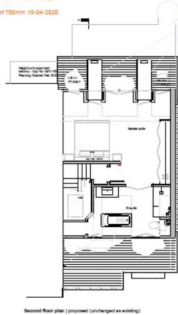
REV A: Balconettes from 2nd floor removed 15-04-2020. No changes to existing 2nd floor plan.
